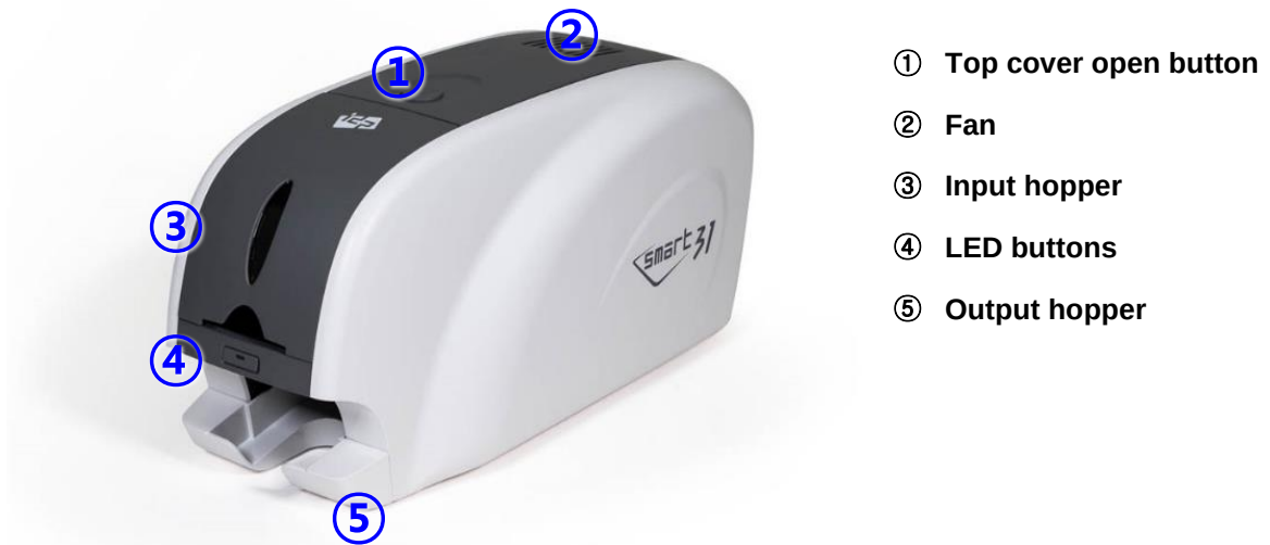
Figure 1 SMART-31 front features
