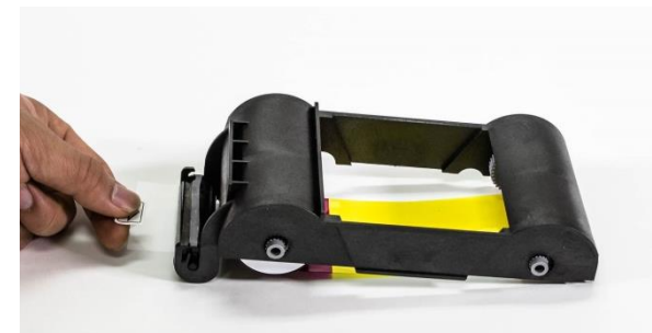
Figure 15 Peeling the protective wrapper
