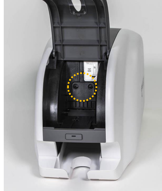
Figure 18 Adjusting the card thickness Device
