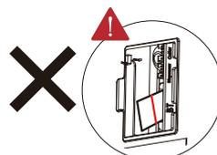
Module not inserted parallel to the mainboard.
