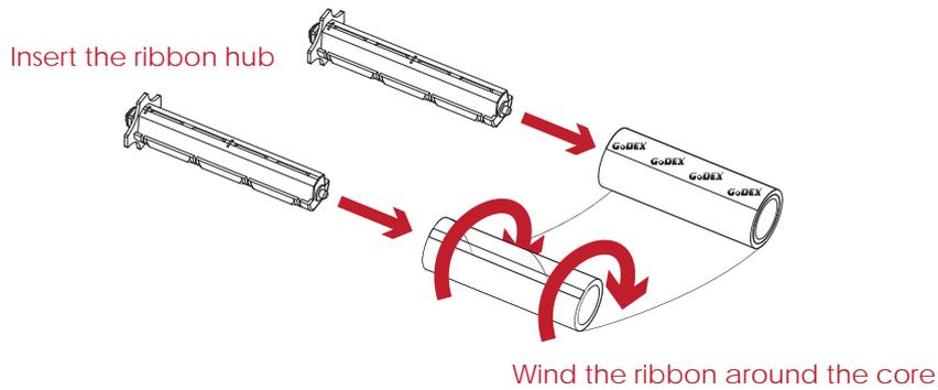
3. A ribbon module is assembled as below.
