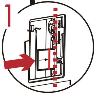
Insert bluetooth module into the slot.
