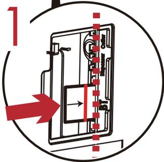
Insert WiFi module into the slot.
