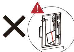
Module not inserted parallel to the mainboard.
