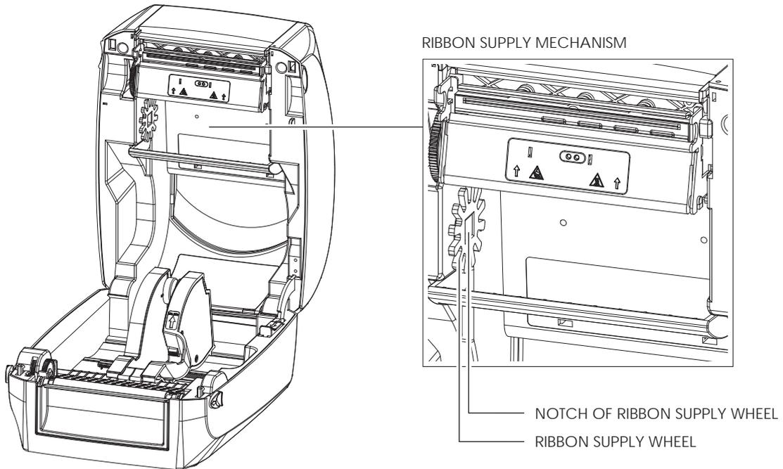
1. Place the ribbon supply module into the printing mechanism. Please the left-hand side of ribbon hub first. Make sure the holder of ribbon hub is inserted into the notch. Then place the right-hand side of ribbon hub.
