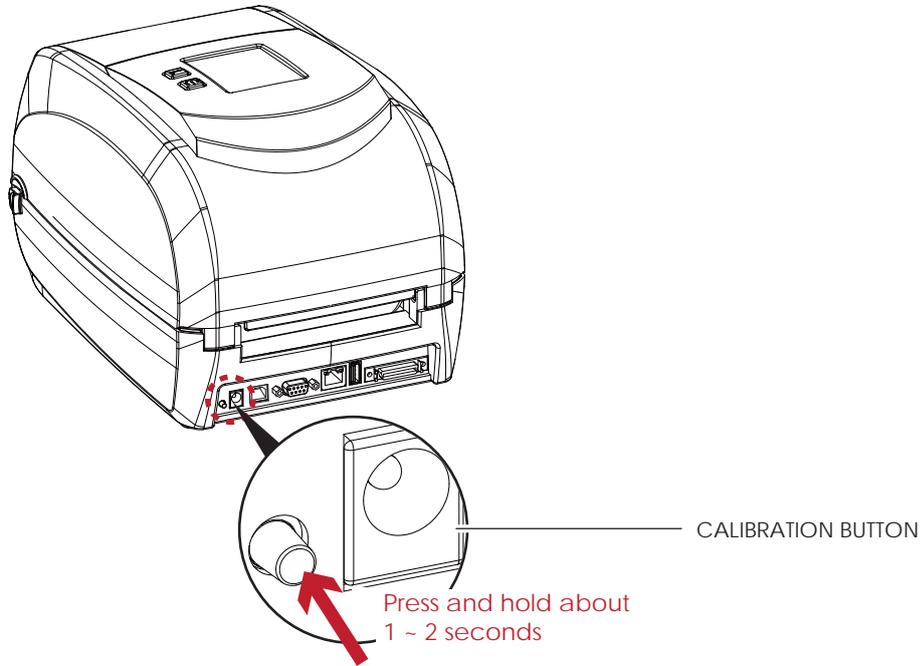
Press Calibration button for 1 ~ 2 seconds, it will make an auto-sensing to calibrate the label's parameters.
