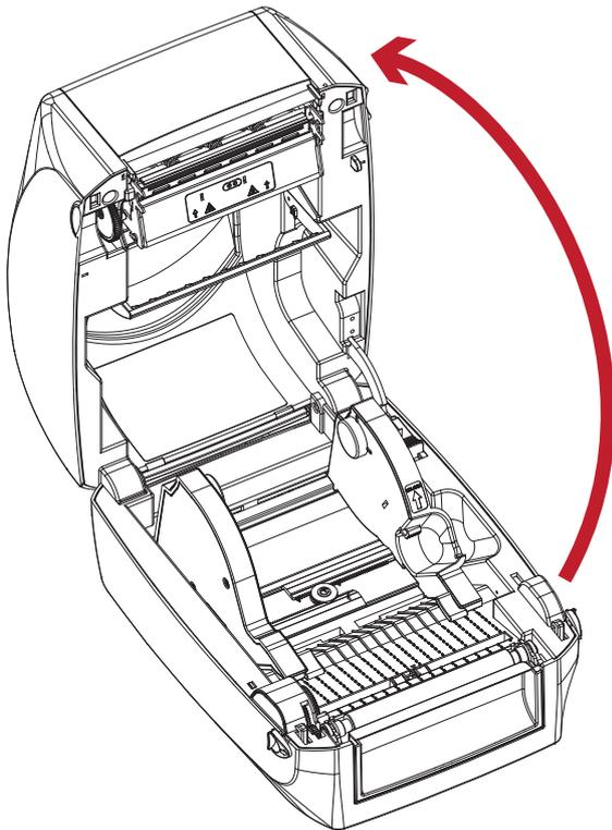
The printing mechanism is lifted up with the printer cover
