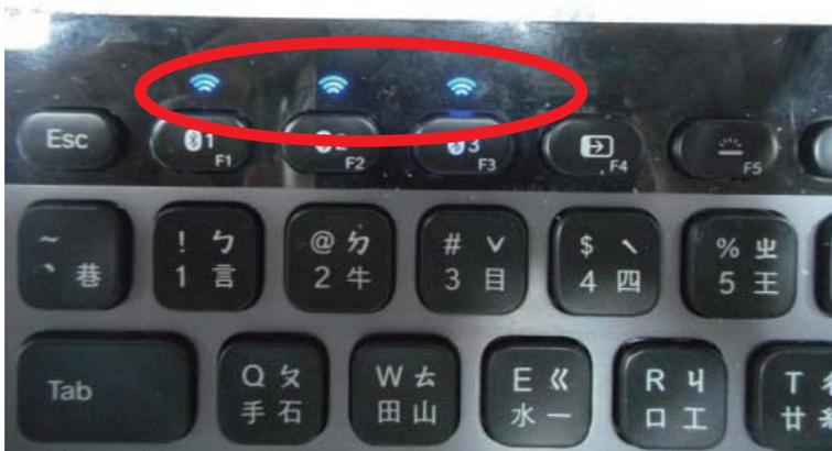
Step 3. The indicator will stop flashing if the Bluetooth keyboard connects to printer properly.
