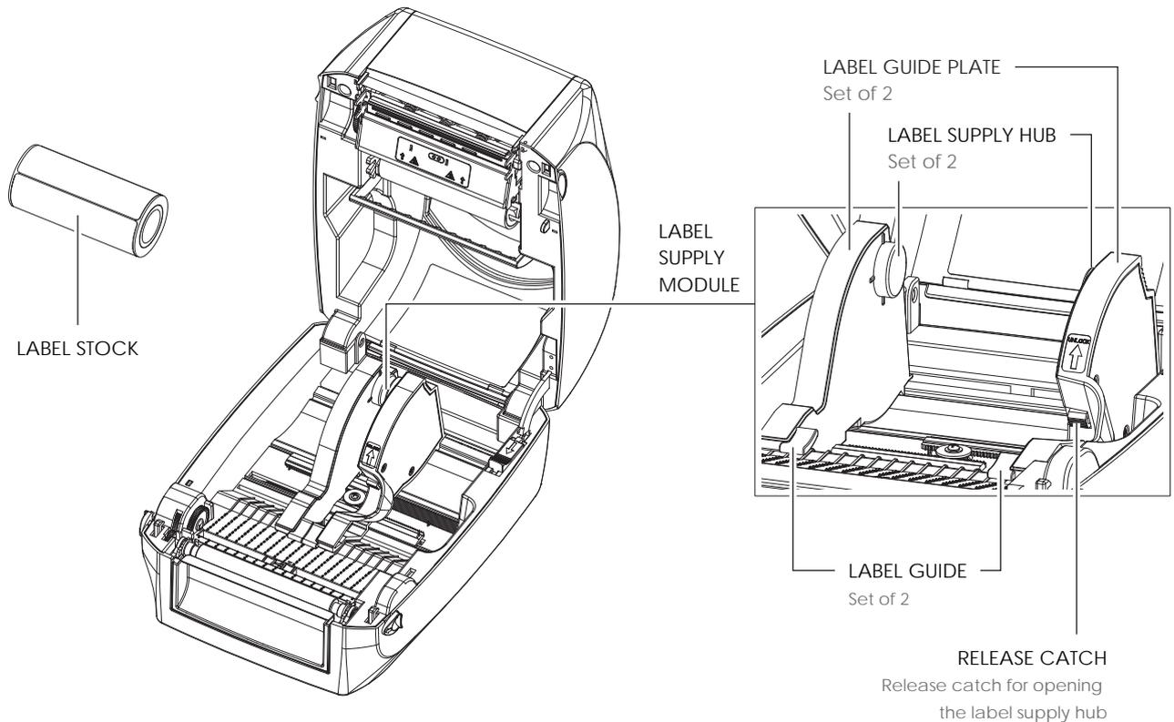
1. Unlock the ribbon catch and pull to open the label guide plate.
