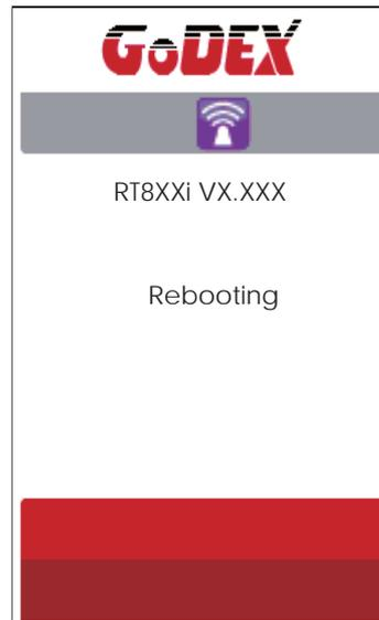
Step 12. If the Wi-Fi Icon turns purple, it means the printer is connected to a Wi-Fi device
