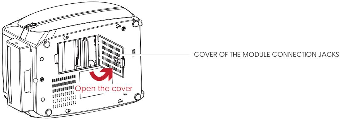
6. Plug the connector for the cutter to the jack.
