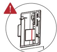
Module not completely inserted.
