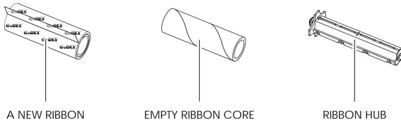
1. Attach the ribbon to the empty ribbon core with the adhesive strip at the end of the ribbon.
