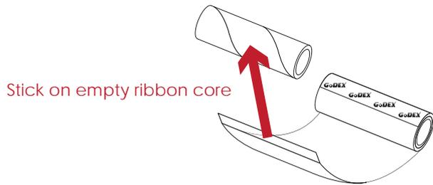
2. Insert the ribbon hub into empty ribbon core and new ribbon. Wind the ribbon around the empty ribbon core for 2 to 3 circles.
