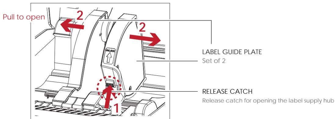
2. Place the label stock on label supply hubs. Make sure the label stock is aligned to both hubs. Adjust the label guide plates to fix the label width. Remember to push the release catch when moving the label guide plates.
