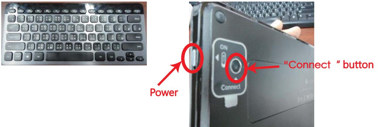
Step 2. The indicator at the upper left corner of Bluetooth keyboard will flash blue when it has been detected.
