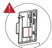
Module not completely inserted.
