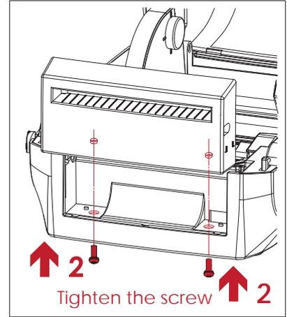
3. Place the platen back to the printer and lock the clips.
