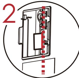
Push the module till the indication line aligns to the edge of mainboard to avoid signal error.
