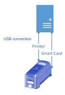
The smart card reader has its own USB connection and communicates directly to the personalization application, usually through a PC/SC interface.
