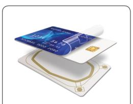
**FARGO High Definition Printing™** (HDP\*) technology delivers superb image quality on smart cards. HDP Film conforms to the uneven surface created by embedded electronics.
